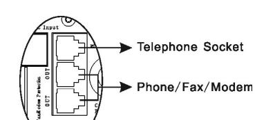
NOTE: This connection is optional but highly recommended as phone/fax/modem lines often carry dangerous surges and spikes. The Unit works properly without a phone/fax/modem connection.
