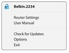
The Belkin Router Manager appears in your system tray (Windows) or menu bar (Mac). Its icon indicates the current status of your Router and also allows you to access your Router's settings to make changes. It also provides quick access to software that came bundled with your Router.
