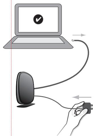
**4** Connect the cable to the Ethernet port on your TV\*, and then plug in the power supply.
