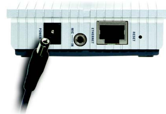
Figure 4-2: Connect the Power Adapter
