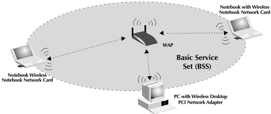
The diagram below illustrates how an WAP acts as a bridge between the wireless BSS and the wired network.
