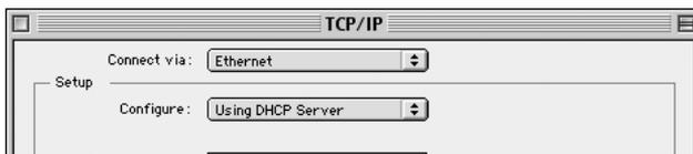
3. At “Configure”: choose “Using DHCP Server”. This will tell the computer to obtain an IP address from the Router.
