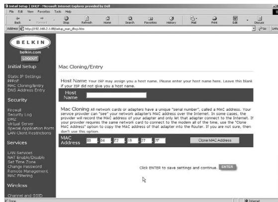
2. Click “Clone MAC Address”. This will clone (copy) the MAC address of the first PC connected to the Router. This will also ensure that the ISP, if it binds your connection to that MAC address, that it will remain active. Click “Enter” to save the settings
