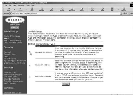
2. Select "Dynamic IP Address" and click "Select". This will tell the Router that the ISP provides a dynamic IP address.
