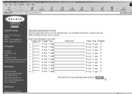
Note: If an application still cannot function correctly after enabling multiple ports via the Special Application screen, you may have to open the client PC for full Internet access using the DMZ Host option.
