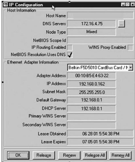
7. This window will provide you with the Adapter Address (also known as the MAC address), the IP Address, Host name (if any) and other network settings. Carefully write this information in the table below, as you may need it later for setting up the Router. For further explanation of what these settings are, see the Glossary of Network Terms in the Appendix of this manual.
