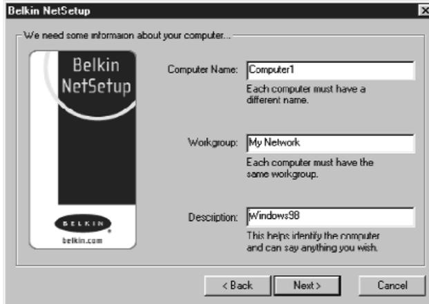
4. In the "Computer Name" field type a name for the computer such as "Computer 1". The name must be different for each computer on the network.
