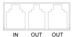
**Note!** This connection is optional but highly suggested as phone/ fax/modem lines often carry dangerous surges and spikes. The UPS works properly without a phone/ fax/ modem connection.
