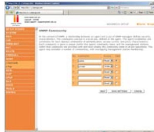
Use the SNMP configuration screen to display and modify parameters for the Simple Network Management Protocol (SNMP). A computer attached to the network, called a Network Management Station (NMS), can be used to access this information. Access rights to the agent are controlled by community strings. To communicate with the VoIP Router, the NMS must first submit a valid community string for authentication.
