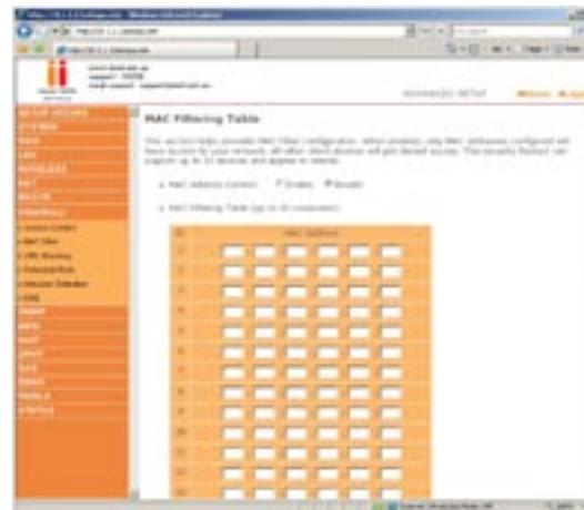
The VoIP Router can also limit the access of hosts within the local area network (LAN). The MAC Filtering Table allows the VoIP Router to enter up to 32 MAC addresses that are allowed access to the WAN port. All other devices will be denied access.
