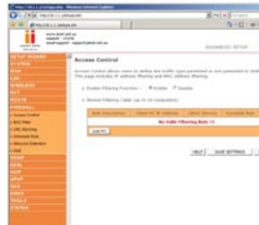
Access Control allows users to define the outgoing traffic permitted or not-permitted through the WAN interface. In the example above, all incoming and outgoing emails are blocked. The default is to permit all outgoing traffic. (See the following page for details.)
