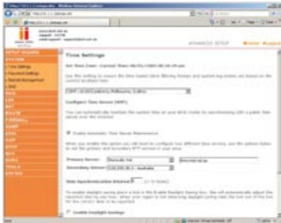
Set the time zone and time server for the VoIP Router. This information is used for log entries and client access control.
