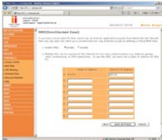
If you have a client PC that cannot run an Internet application properly from behind the firewall, you can open the client up to unrestricted two-way Internet access. Enter the IP address of a DMZ (Demilitarized Zone) host on this screen. Adding a client to the DMZ may expose your local network to a variety of security risks, so only use this option as a last resort.
