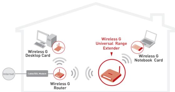
**Note:** Laptops can roam or move between the two wireless coverage areas if the SSID and the parent access point's SSID match.
