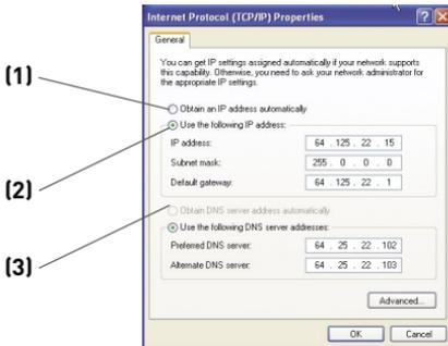
5. If “Use the following IP address” (2) is selected, your Router will need to be set up for a static IP connection type. Write the address information into the table below. You will need to enter this information into the Router.
