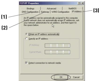
3. If “Specify an IP address” is selected, your Router will need to be set up for a static IP connection type. Write the address information in the table below. You will need to enter this information into the Router.
