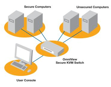
The OmniView Secure KVM Switch lets you safely control up to eight USB computers running on different security levels from a single USB console (4-port model shown).
